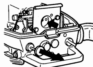
(Fig. 9-14) Checking the choke valve
